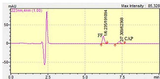
Figure 3. Chromatograms images of standard solutions of FF (3 µg/g) and CAP (1.5 µg/g).
